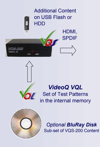
Compact size tool, loaded with unique sophisticated set of static and dynamic test patterns up to 1080p@60fps, ideally positioned for applications in:
